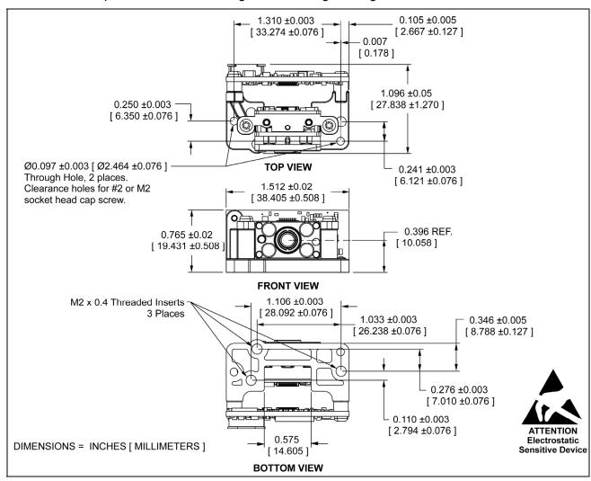
Figure 13. IS4920 / IS4921 Bracketed Decode Engine Dimensions
